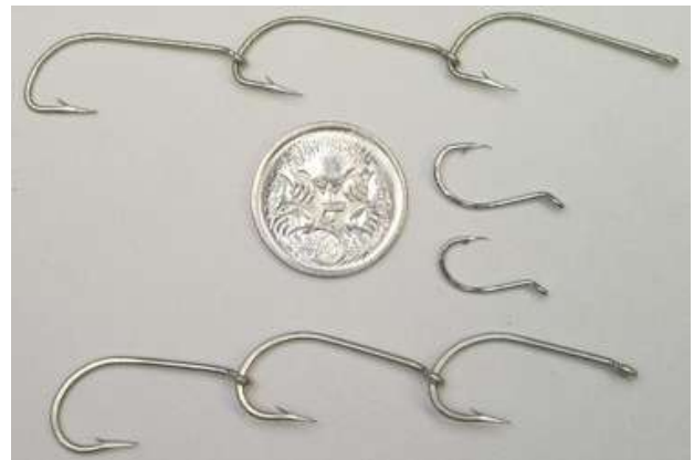
Ganged hooks "Limerick" type on top, stronger "Tarpon" on bottom, for whitebait or bluebait, "suicide or beak" hooks for bait in centre. Size compared with a 5 cent coin
