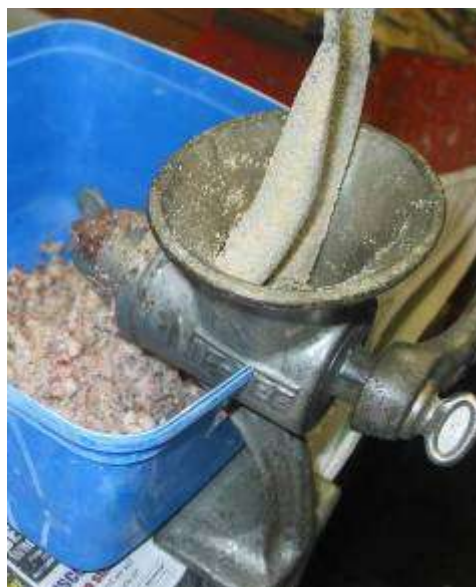
Mincer clamped to a bench with a container to catch the minced fish
